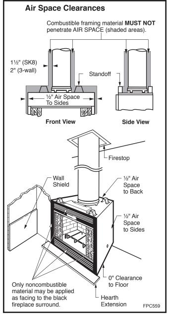
Fig. 21 Minimum clearances to combustibles.
